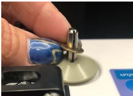
Add 1 thin washer to bobbin post if you have an L bobbin ONLY! M bobbins will not need the washer
