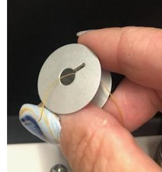
Feed thread through bobbin slot or wrap around bobbin 4-5 times counterclockwise
