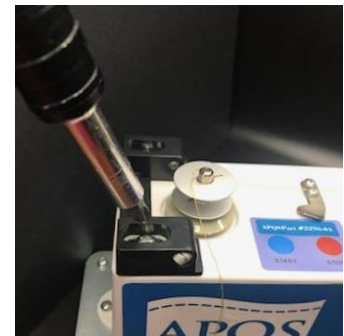
Sensor adjustment screws - one on each side of sensor housing
