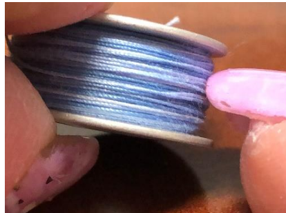
Thread should feel firm, not spongy on bobbin
