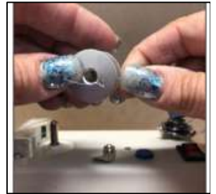
4. Adjusting sensor position to set for bobbin size.
