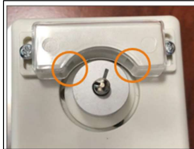
6. Bobbin Fill Level Sensors “read” across outer edge of thread on the bobbin.
