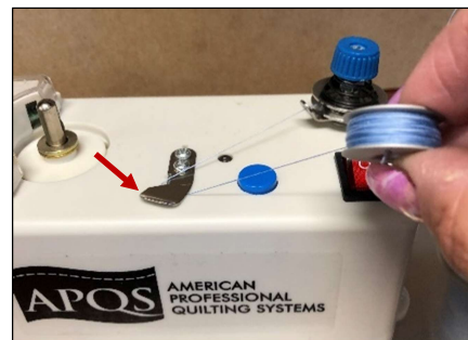
16. A thread cutter IS included on the bobbin winder housing.
