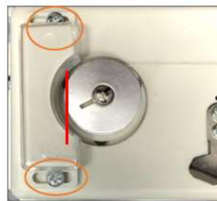
9. Preliminary setting for “M” size bobbins.
