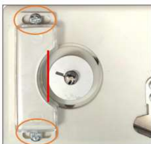
8. Preliminary setting for “L” size bobbins.
