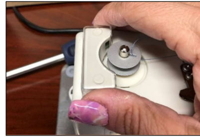
10. Adjusting sensor position to set for bobbin size.
