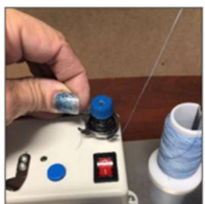
2. Place thread through the first guide, around the tension discs counterclockwise and through the second guide.
