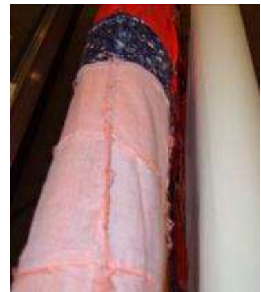
Horizontal seams should not twist. Photo above is showing twisting.
