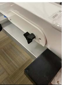
C. Secure the Lower Frame Belt Bracket with the supplied knob screw. Alternatively, you can reinstall the laser post and nut instead of the knob.
