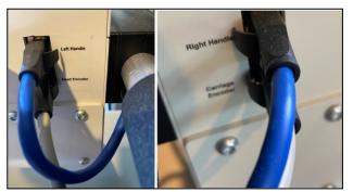
A. Unplug both the left- and right-handle blue cables from the rear of the machine.
