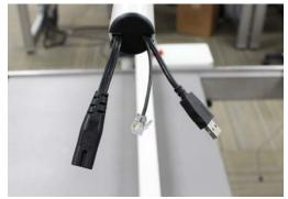
F. Arrange the three wires so the power cord IS facing the left side. The USB cable and switch cable should be facing the right side.
