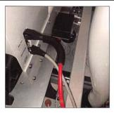
B. The photos above show the Quilt Path Aux Line cable (red) mounted in the clamp and the correct orientation for the cable – this should be done to the Encoder cable (grey) as well.
