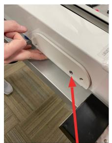
B. Slide the Lower Frame Belt Bracket in between the sewing head and carriage as shown above. Line up the second hole from the right with the laser post hole.
