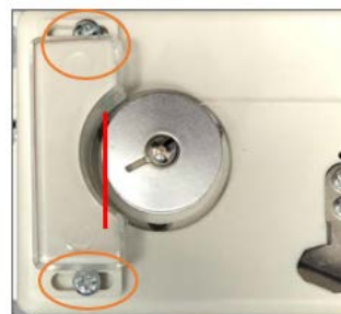
9. Preliminary setting for “M” size bobbins.
