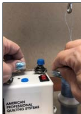
3. Pull on thread to seat between tension discs.
