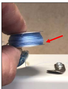
14. Filling towards bottom? Remove one thin washer.
