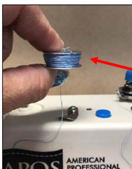
13. Filling towards top? Add one thin washer.
