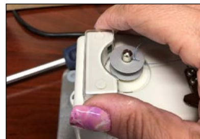
10. Adjusting sensor position to set for bobbin size.
