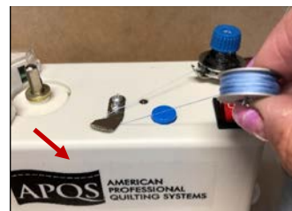
16. A thread cutter IS included on the bobbin winder housing.
