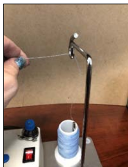
1. Pull thread up and over the thread stand from the right to the left.
