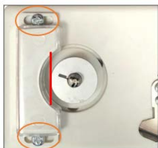
8. Preliminary setting for “L” size bobbins.
