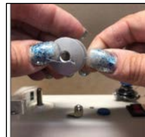
4. Adjusting sensor position to set for bobbin size.
