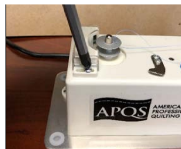
7. Sensor adjustment screws – one on each side of the sensor housing.
