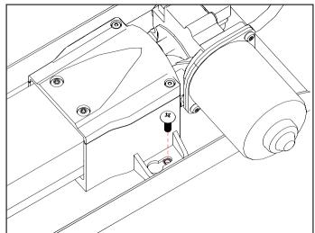
Place the pump with the attached mounting bracket on the floor near the middle of the table as shown. (Place the pump so that the motor on the pump is toward the left leg when standing on the pantograph side of the table.)
