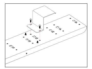
Bolt the cylinder mounting brackets to the four lift cylinders. Use (4) 5mm x 10mm screws and (4) 5mm washers on each mounting bracket as shown. Position the bracket so that the "fork" points away from the lift cylinder.
