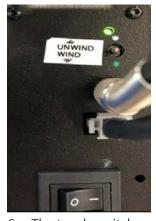
6. The toggle switch on the motor controller can be used instead of the foot pedal.
