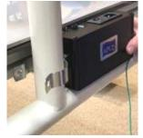
5. Slide the bracket onto the right table leg.
