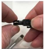
4. Replace the blown fuse with the new fuse and reinsert the fuse holder into the motor control box.
