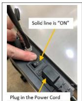
4. Insert the power cord. Press the switch to the solid line to turn on the Automatic Quilt Advance.
