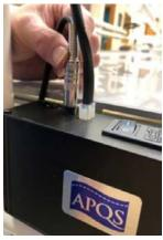
Plug the foot pedal into the pedal jack on the motor controller.
