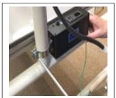
3. Hold the controller in place and tighten the bracket screw.
