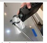
Remove the screw from the mounting bracket.
