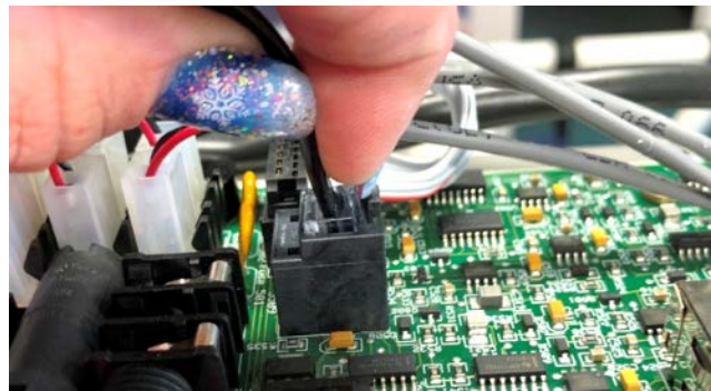
Remember to reconnect cable to thread break sensor before reinstalling cover.
