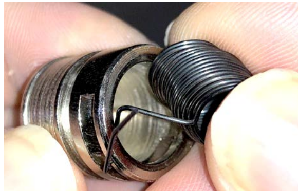
Slide bottom of spring towards base.
