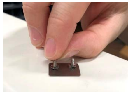
Add 3 wave washers to each screw.
