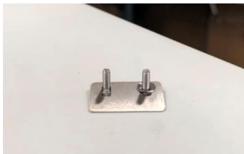
Add 3 wave washers to each screw.
