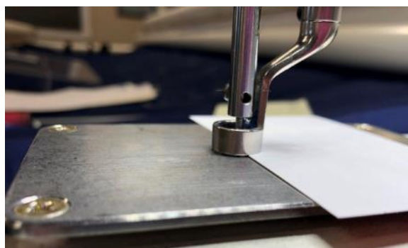
Checking hopping foot height.
