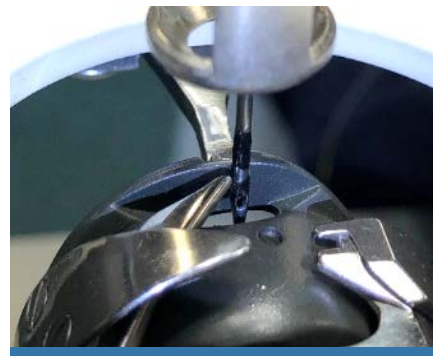
Needle brought up to locate silver stripe on needle scarf.
