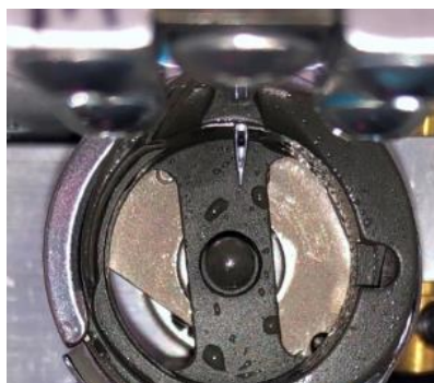
Needle Depth – Style "L" Hook Assembly
