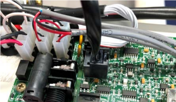
Wire connection for thread break sensor in center of circuit board.
