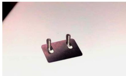
First blade on screws flat side up.
