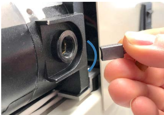
Curvature in end of motor brush
