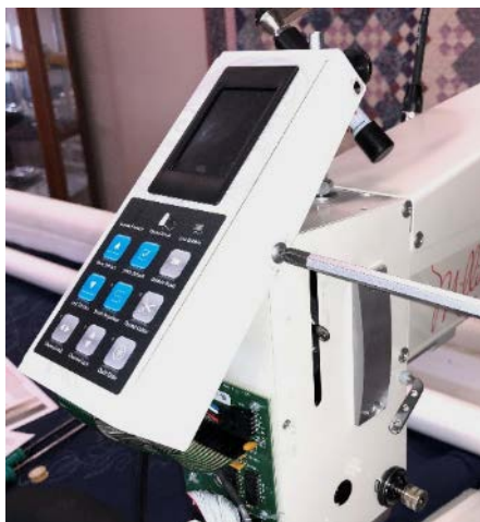
Use 1 Phillips screw to hold front cover on machine.
