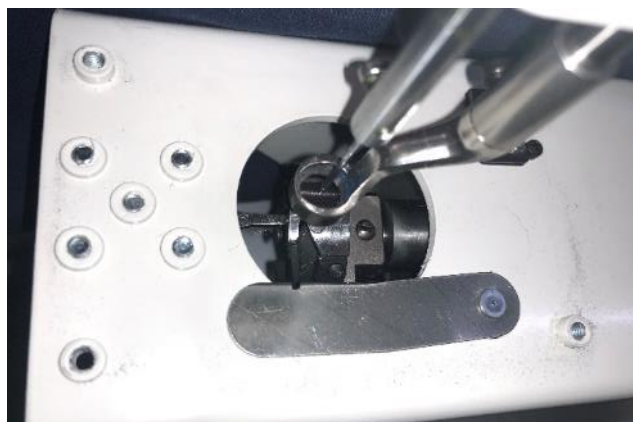
Spacers are permanently attached to machine.
