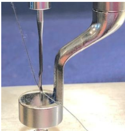
Needle viewed from thread path side of machine.
