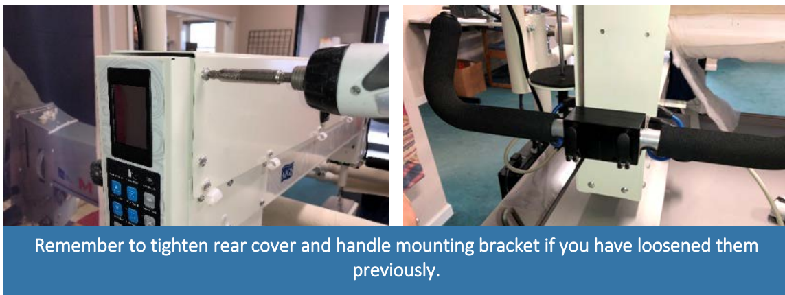
Tighten screws securely – DO NOT OVER-TIGHTEN!
