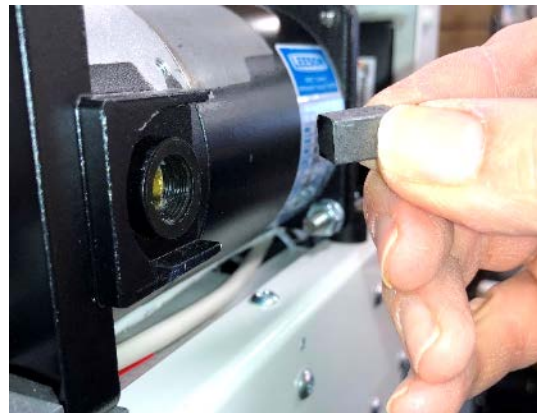
Incorrect motor brush alignment.
