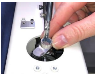
Push leading edge of puller arm into opening on throat of machine.
