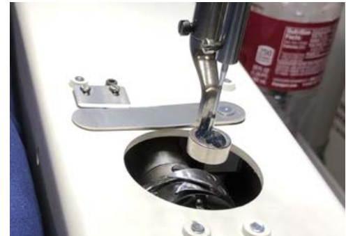
Puller arm caught on edge of cutting blades.
