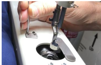
Remove 2 screws holding blade assembly on machine.
