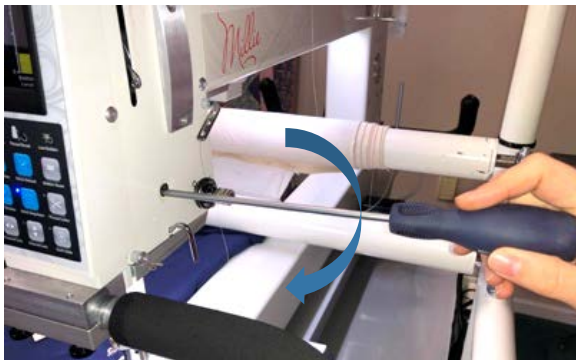
Tighten clamping screw while holding hopping foot in desired position.
