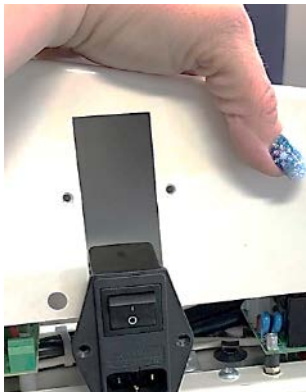
Cover clearance around power cord module.
