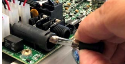
Squeeze metal side clips to hold fuse in position for reinstallation in board.
