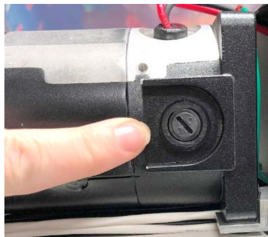
Correct brush cap position.
