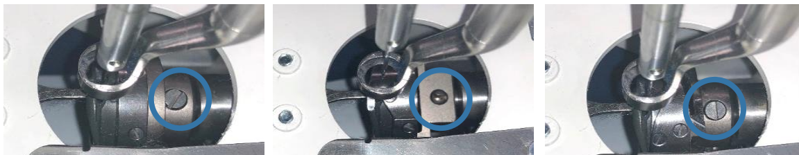
Loosen 3 screws that hold hook assembly onto machine.
