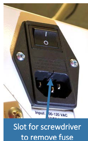
Use screwdriver to pry fuse drawer out of power
