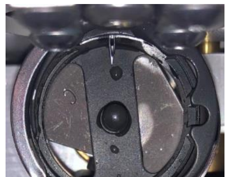
Needle Depth – Style "M" Hook Assembly
