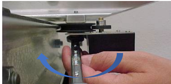
Loosen mounting bolt with 7/16" wrench.
