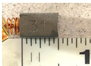
Measuring motor brush length
