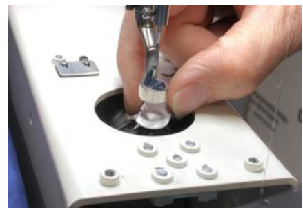
Pull up on leading edge if it is too low to clear cutting blades.
