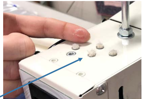
Oil residue on fingertip = NO OIL NEEDED
