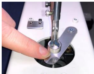
Push down on leading edge if it is too high to clear cutting blades.
