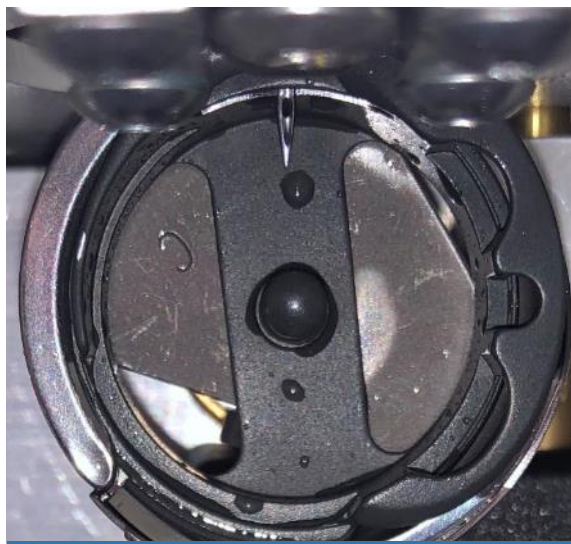
Needle Depth – Style "M" Hook Assembly
