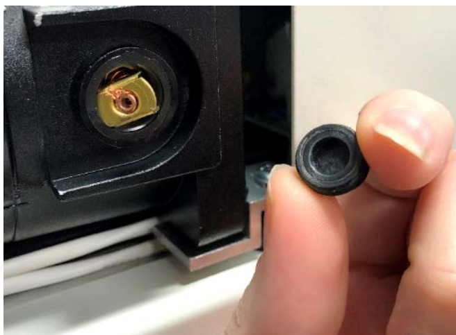
This side of brush cap goes inside the motor.
