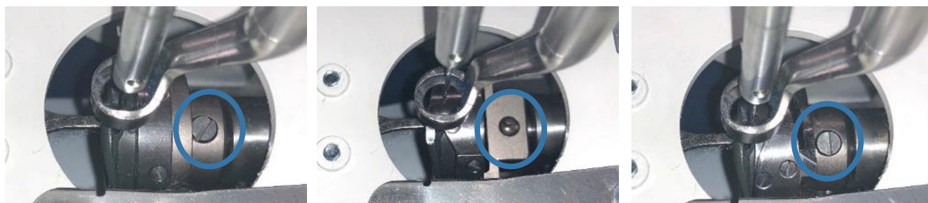
Tighten 3 screws that hold hook assembly onto machine. On Style “L” Hook Assemblies – DO NOT OVER-TIGHTEN the screw in middle photo!
