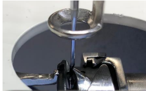
Hook point touching side of needle to allow for hook finger positioning.
