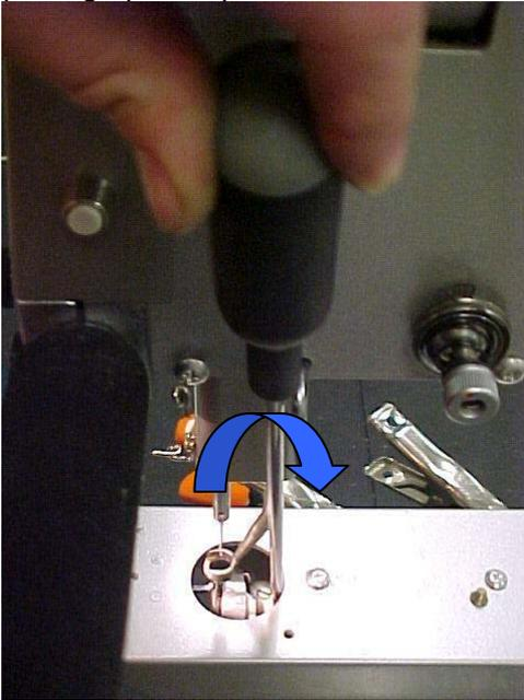
Then, come up from underneath the machine with 2 long handled screwdrivers, and put the blades in the space created, then twist the screwdrivers to 'walk' the old hook assembly off the shaft. **DO NOT USE THE FRAME OF THE MACHINE TO PULL THE OLD HOOK ASSEMBLY OFF THE SHAFT!!!** You greatly increase the risk of un-seating the brass bushing around the hook shaft and damaging the gears inside the gear box.
