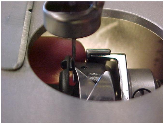
Install the hook finger as shown below, with space between the end of the hook finger and the face of the bobbin basket, but do not tighten down the Phillips screw holding the finger yet – the finger placement will be adjusted later. The hook finger should be snug enough to hold the basket from spinning, but the exact position is not critical at this point. Now, you can begin the timing process!
