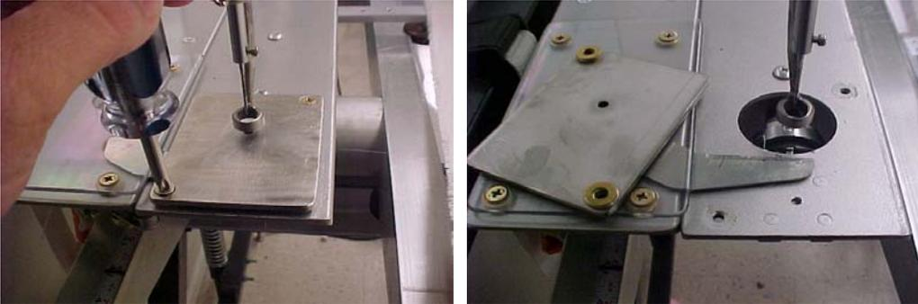
Remove hook finger using Phillips screwdriver.
