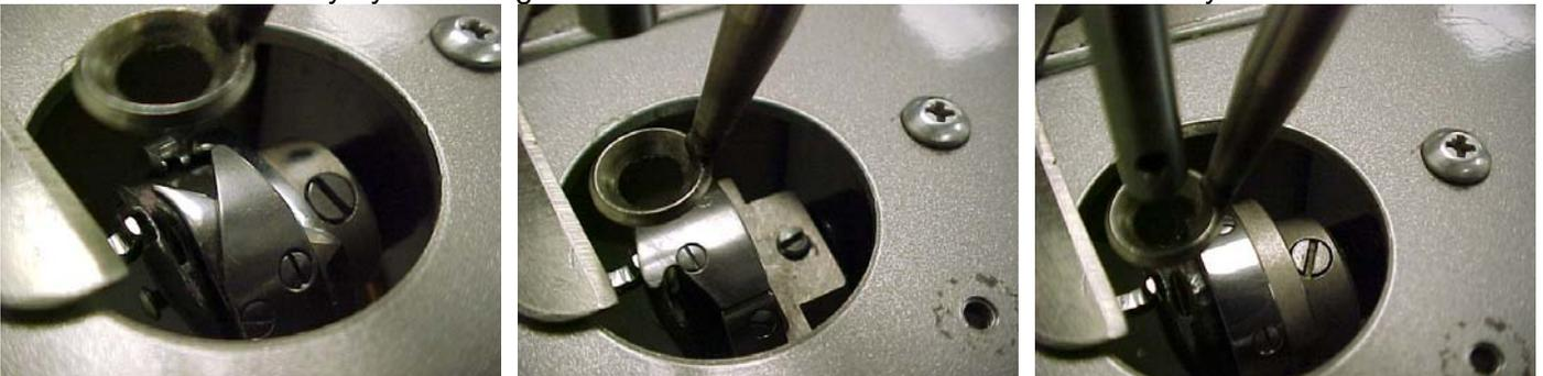
The hook assembly will be difficult to remove, because the screws have scarred up the hook shaft. Use the following process to remove the old hook: Looking down through the hole in the throat of the machine, locate the black locking collar that is on the shaft behind the back of the hook assembly. This space will be used for removing the hold hook assembly.
