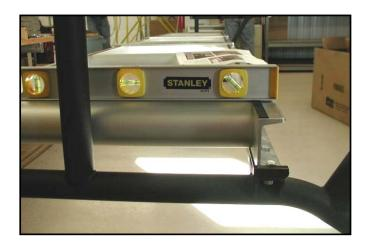
Place a level directly on top of the table frame, across the two aluminum rails near the end of the table (parallel to the leg).
