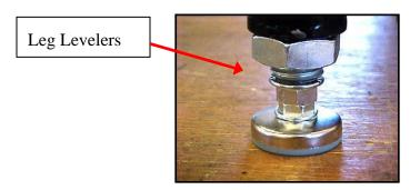
To adjust leg levelers, first loosen the large jam nut directly underneath the leg; use the large box end leg wrench found in the accessory box.
