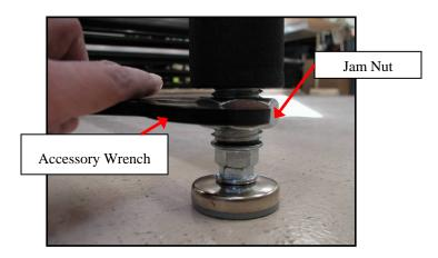
Next, use a 3/4" box end wrench on the smaller nut as shown below to adjust the leg's leveler pad. Turning the smaller nut clockwise causes the table to raise up (you're screwing the leg out farther); turning the small nut counterclockwise lowers the table. <u>The table legs are adjustable up to a maximum of 9 inches.</u>
