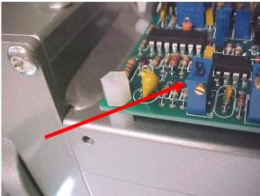
Gently turn the screw on #8 clockwise (right) to slow down the positioning speed. Counterclockwise (left) will increase the positioning speed. Note: If the speed is set too slow, the needle will not position correctly or may not move at all. If the speed is set too fast, the needle may continue to move up and down and not stop at all. You may need to rotate the adjusting screw 1 – 2 revolutions as needed. Only adjust #8 do not adjust any other screws.
