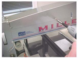
Remove the 2 front screws on each side of the top cover as shown.
