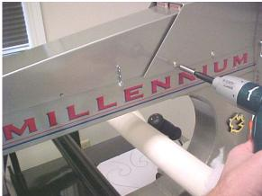
Loosen the 3<sup>rd</sup> screw on each side, do not remove. Start the machine in manual mode at about ½ speed and let it warm-up for 5-7 minutes before proceeding.
