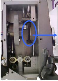
Once the washers are cleaned of thread, gently push the black arm back towards the flywheel. Before tightening the set screw on the flywheel, check to be sure the black arm isn't pushed back so far that the gold washers can't spin on the shaft. Tighten the set screw once a satisfactory position has been attained. If you used WD-40 to help loosen the thread, be sure to put a drop of oil on the washers to lubricate the area before running the machine.
