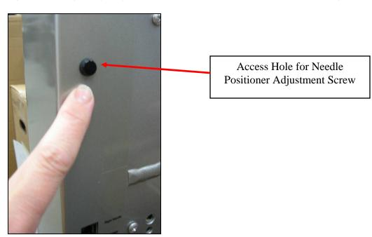
The "Adjustment Screw" is located inside the access hole on the right rear of the sewing head (when viewed from the pantograph side)
