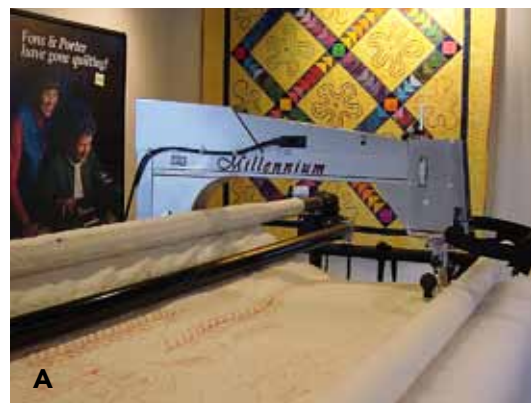
Best tension is achieved by moving a longarm machine from left to right when standing on the needle side of the machine.
