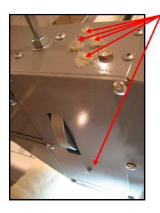
Rub your finger across each of the 5 oiling wicks; it should be wet with oil. If any wick is dry, add two drops of oil to that wick.
