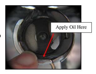
Keep the rag out of the way of moving parts and start the machine again using the "command-blue" button sequence on the RIGHT handle. Allow the machine to run for 10-15 seconds so that the oil can be distributed in the hook assembly.
